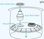
To assemble, place the Auto Skim Valve into the opening in the new Vacuum Plate and attach you hose. If you notice a slurping sound, attach the Anti-Vortex Disc over the valve inlet. Place the entire unit in the skimmer box.
